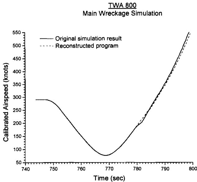
As seen in the plots above, the reconstructed code could not reproduce the flight path from the Addendum II to Main Wreckage Flight Path Study past the time of the outboard wing panel failure. This indicates that the preserved version of the TWA 800 aerodynamic code was edited for further iterations after the simulation runs used in Addendum II.
